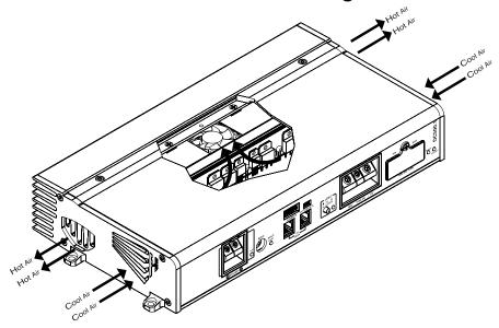
Here is an unfortunate fact: Generating power creates heat. As ZAPCO has learned to put more power into a smaller package, the management of thermal properties has become increasingly important.
